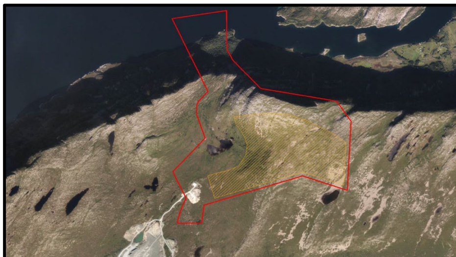
Figure 7. The existing quarry at Sætreffjellet to the left (south). Outlined in red is the plan boundary of the Aksla quarry with the extraction area in yellow, and stone crushing plants, industrial area and a shipping port to the north. Note that the steep mountain side is partly hidden in shadow.
